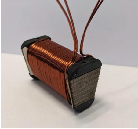
FIGURE 3: Stator tooth with bifilar winding.
